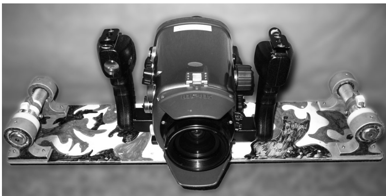
Fig. 1. Pair of green, underwater laser pointers mounted in parallel to an underwater video housing
